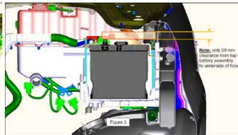
Figure 3: Section View at LH Battery
