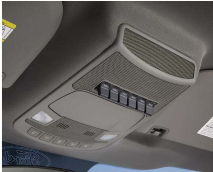
The Ford Upfitter Switches are optional overhead console mount switches (Option Code 66S) that control under hood mounted relays (see Upfitter Relay Box section in this BBLB). All fuses are located in the Upfitter Relay Box.
