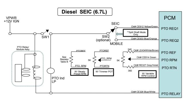
\*\* For Split Shaft operation, both PTORS1 & PTORS2 must have line voltage applied.
