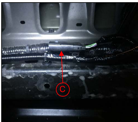
Figure 2: Box delete harness installation – jumper harness shown installed
