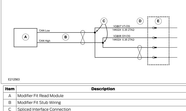
D Ford CAN Loop Wire - CAN High is the Gray/Orange wire. CAN Low is the Violet/Orange wire
