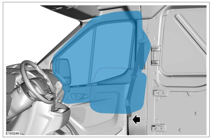
MARNING: Do not drill in Right Hand/Left Hand side retractor assy area.
