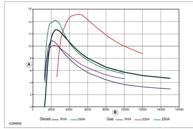
Diagram E284685 shows the torque in Nm which is required to drive the alternator at full output. The vertical axis (A) shows the torque (Nm) and the horizontal axis (B) shows the alternators revolutions per minute (rpm). **NOTE:** For equivalent engine revs per minute (rpm), the alternators revolutions, axis (B) should be divided by the following factor: 2.69 for 3.2L diesel.
