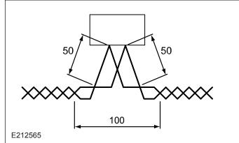
It is allowed to connect modules to the backbone using a series chain method instead of a stub. If the series chain method is selected, the untwisted wire on each side of the double crimp in the connector cannot exceed 1.96" (50mm). See figure E212565
