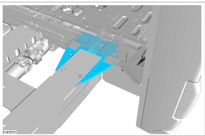
Do not drill or cut in the reinforcement plate on single chassis cab/cutaway vehicles.
