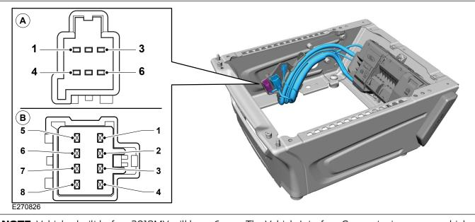
**NOTE:** Vehicles built before 2018MY will have 6 way- connector A and vehicles built starting 2018MY will have 8 way - connector B. See figure E270826 for location and the following table for signals.
