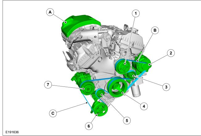
Description Item 1 Water Pump 2 Alternator 3 **Belt Tensioner** 4 Crankshaft Pulley 5 Belt Tensioner б Power Steering Pump 7 Compressor А Engine Top Cover Primary FEAD Belt В С Secondary FEAD Belt
