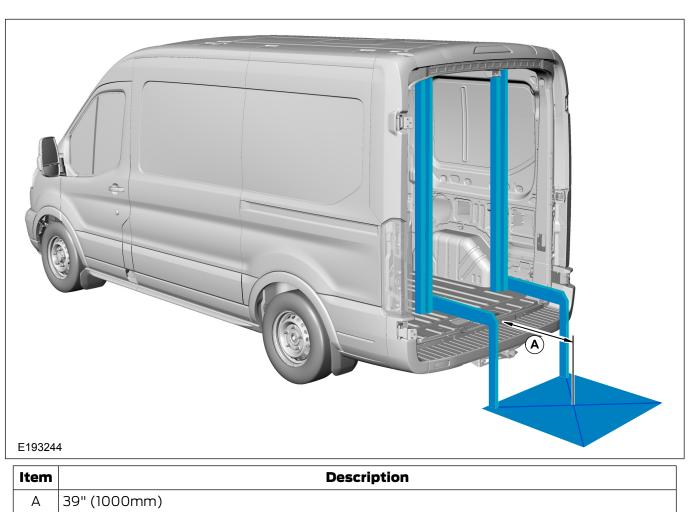
It is recommended to fix lift framework on bottom and on top side by using reinforcing plates and through bolts. It is also recommended to design and/or locate the reinforcing plates in a way that load can be routed into adjacent reinforced body structure.
