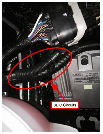
**TRANSIT ENGINE COMPARTMENT** • 3.5L / 3.7L SEIC Circuit Location - found underhood, taped to harness next to Engine Junction Box
