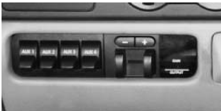
Finished installation of Upfitter Switches with Trailer Brake Controller
