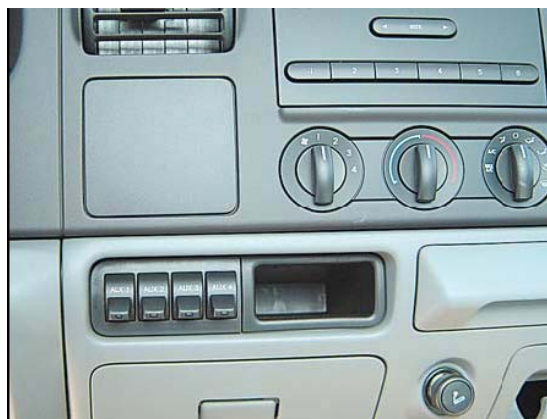
Finished installation of Upfitter Switches without Trailer Brake Controller (empty pocket)
