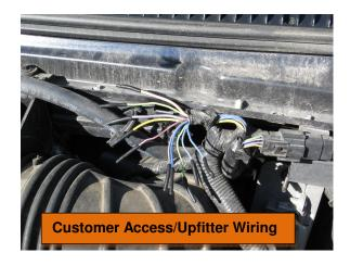
The two pass-thru wires are part of the same modified vehicle wiring kit as prior years. Located at the 4-pin connector in the harness below the cowl, outboard of the brake master cylinder, as shown. Mating pigtail connector, 4C24-14A411, found in dunnage.
